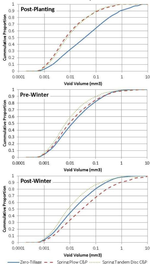
Figure 4 - Cumulative size distribution of resolvable pores, with volumes ranging from >8 to <100,000 voxels.
